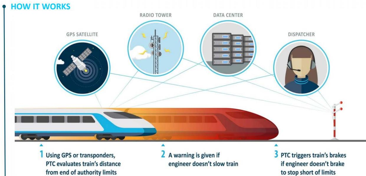
*For example, PTC can force a train to stop before it passes a signal displaying a stop indication, or before running through an improperly lined switch, averting a potential collision.*
